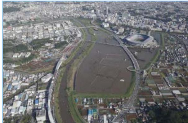
Flood adjustment by Tsurumi River multipurpose water reservoir
