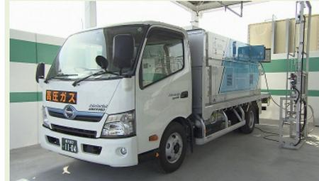
A simplified hydrogen-filled car was first introduced in Japan. Hydrogen compressed to 45 MPa is brought to the customer and fueled in the site.
