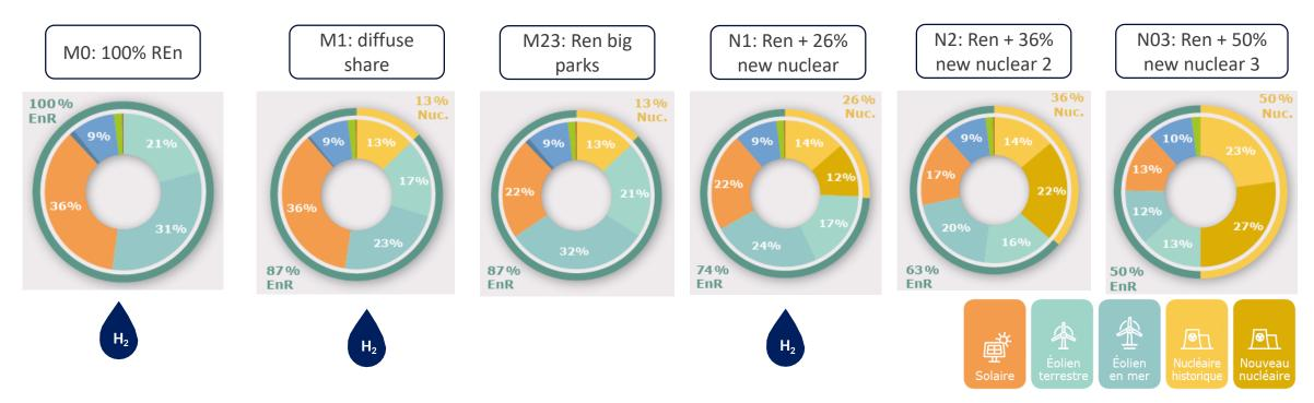
RTE anticipates several degrees of integration of a "low-carbon hydrogen system" combining hydrogen production, storage and transport, notably as a **means of flexibility** essential to the M0, M1, M23 and N1 scenarii from 2040.
