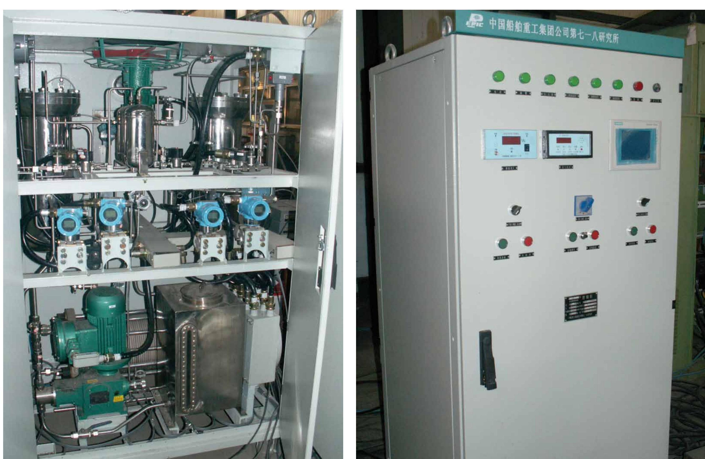
The first box type 1.0 Nm 3 /h alkaline and SPE (solid polymer electrode) water electrolysis system in China
