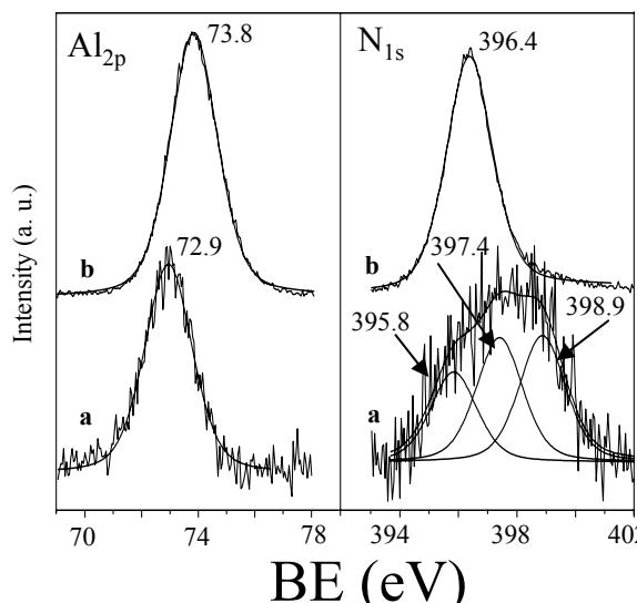
XRD, FTIR and XPS investigations reveal stepwise phase changes and the development of a new ternary Li-Al-N-H compound. Three N states were identified.
