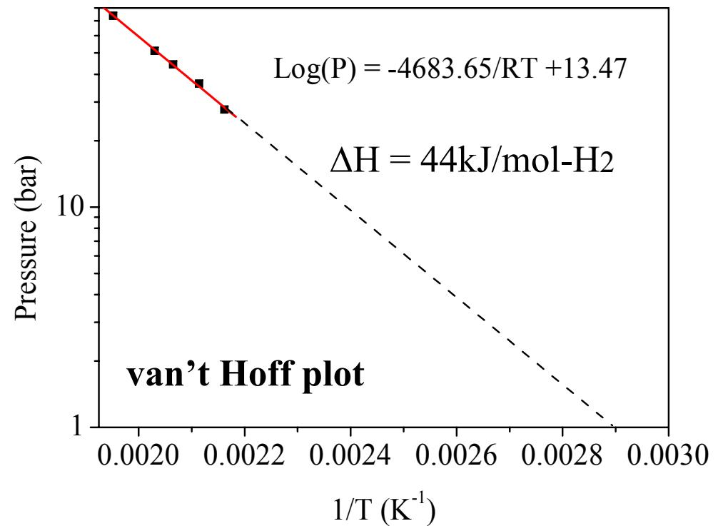
Thermodynamic analysis shows the operation temperature could be below 363K.
