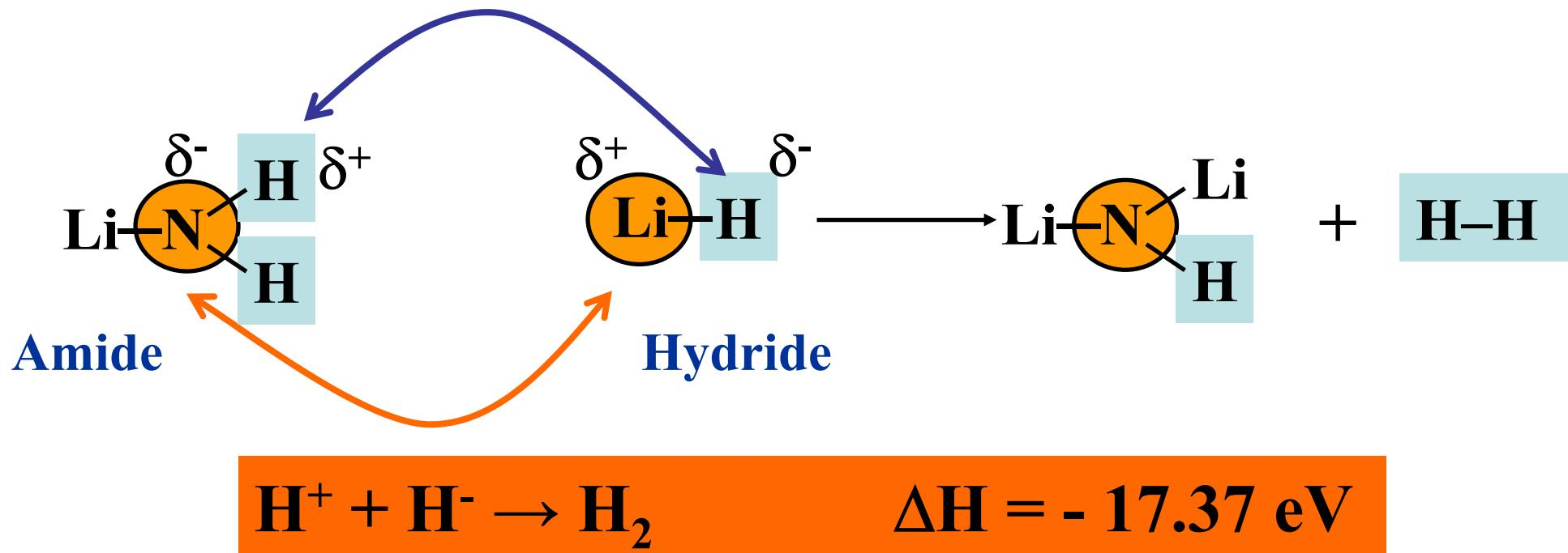
The abnormally high potential for the combination of  $\text{H}^+$  and  $\text{H}^-$  to  $\text{H}_2$ , and the Columbic attraction between N and M are likely to be the driving forces!
