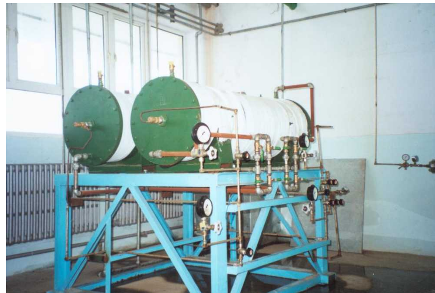
MH hydrogen storage units for hydrogen purification and compression
