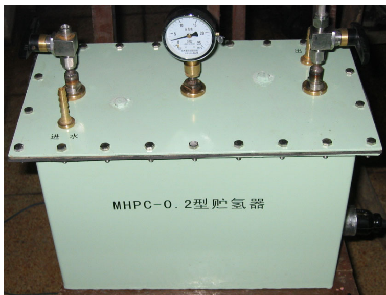
Mini-type MH hydrogen storage-purification unit
