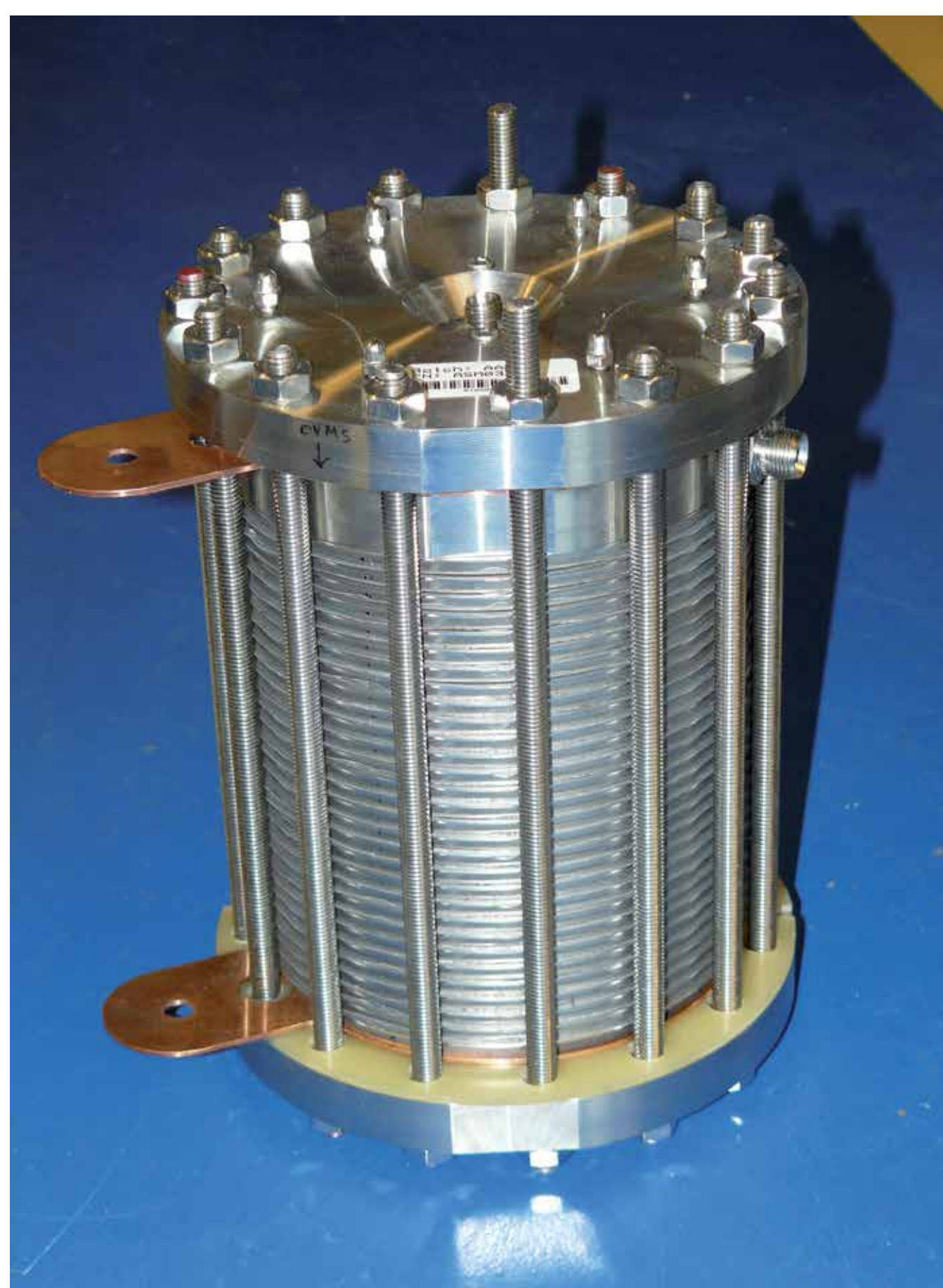
The 29-cell PrimoLyzer stack with a production capacity of 1 Nm 3 H 2 /h.
