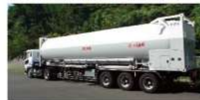
Type ISO 40ft-type container Volume 45.6m 3
