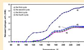
The amount of re-absorbed hydrogen drops to 2.2 - 2.6 wt% after the first desorption.
