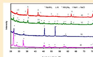
XRD patterns of 4 mol% ZrCl<sub>4</sub> doped NaAlH<sub>4</sub>, a) as-received NaAlH<sub>4</sub>, b) milled 4 mol% ZrCl<sub>4</sub> doped NaAlH<sub>4</sub>, c) rehydrated 4 mol% ZrCl<sub>4</sub> doped NaAlH<sub>4</sub> at 120 °C, d) dehydrated 4 mol% ZrCl<sub>4</sub> doped NaAlH<sub>4</sub> at 280 °C.
