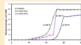
Doping transition metal on milled LiAlH<sub>4</sub> decreases temperature of decomposition and increases the kinetics. Again, different desorption behaviors can be observed.
