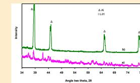
XRD patterns of a) as-received LiAlH<sub>4</sub>, b) dehydrated LiAlH<sub>4</sub> at 170 °C.
