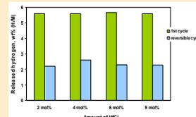
Amount of released hydrogen and absorbed hydrogen as a function of HfCl<sub>4</sub> amount.
