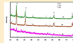
XRD patterns of a) as-received LiAlH<sub>4</sub>, b) dehydrated 4 mol% ZrCl<sub>4</sub> doped LiAlH<sub>4</sub> at 150 °C, c) milled LiAlH<sub>4</sub> by using centrifugal ball mill.
