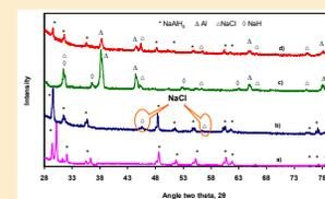
XRD patterns of 4 mol% HfCl<sub>4</sub> doped NaAlH<sub>4</sub>, a) as-received NaAlH<sub>4</sub>, b) milled 4 mol% HfCl<sub>4</sub> doped NaAlH<sub>4</sub>, c) rehydrated 4 mol% HfCl<sub>4</sub> doped NaAlH<sub>4</sub> at 120 °C, d) dehydrated 4 mol% HfCl<sub>4</sub> doped NaAlH<sub>4</sub>.
