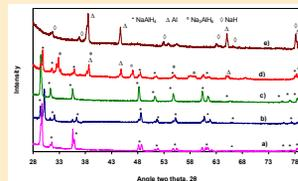
XRD patterns of undoped NaAlH<sub>4</sub>, a) as-received NaAlH<sub>4</sub>, b) milled NaAlH<sub>4</sub>, c) dehydrated NaAlH<sub>4</sub> at 120 °C, d) dehydrated NaAlH<sub>4</sub> at 196 °C, e) dehydrated NaAlH<sub>4</sub> at 280 °C.
