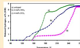
Doping transition metal on milled NaAlH<sub>4</sub> decreases temperature of decomposition and increases the kinetics. Different desorption behaviors can be observed.
