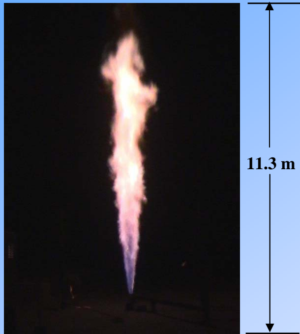
Nighttime photograph of 413 bar (6000 psig) large-scale H 2 jet-flame test ( d_j = 5.08\text{mm} , L_{\text{vis}} = 10.6\text{ m} ) from Sandia/SRI tests.
