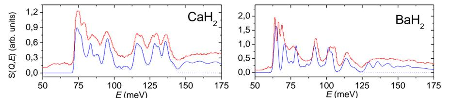
Fig. 2: measured INS spectra of alkaline earths hydrides and *ab-initio* calculations
