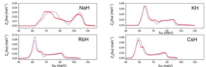
Fig. 1: measured INS spectra of alkali hydrides and *ab-initio* calculations
