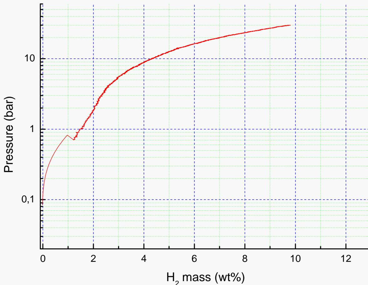
Li<sub>3</sub>N<sub>16</sub>C<sub>36</sub>H<sub>36</sub>O<sub>4</sub>Ti P<sub>max</sub>=30bar, Flow=20ml/min, Temp=285°C,
