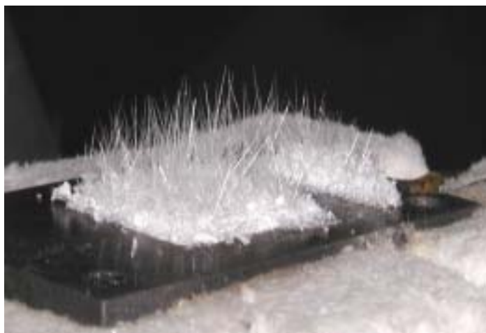
Growth of ammonia borane needles at 80°C
