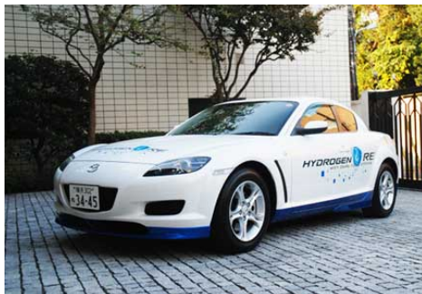
10 Mazda RX-8 Delivery in 2009/2010 Flexifuel wankel engine Range: 100 km H 2 , 50 km gasoline
